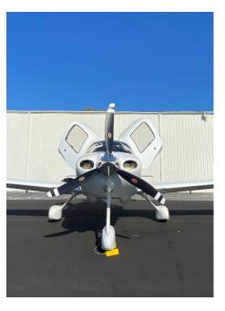
Avoid taxiing an airplane near uneven pavement or unimproved surfaces. Rock can be sucked up and cause damage to the propeller or airframe. Uneven pavement or sloped ground can potentially cause a propeller strike and cause significant damage.
