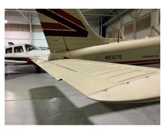
A combination of neutral trim indication in the cockpit/neutral control wheel should result in the anti-servo tab being flush with the trailing edge of the horizontal stabilator.
