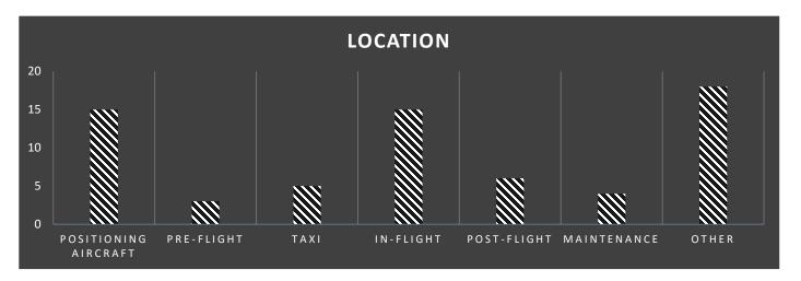
Report data indicates a strong trend of issues during the positioning of aircraft on the ground. Most reports are related to placing aircraft in improper parking spots in the hangar or on the ramp, where they lead to potential damage.
