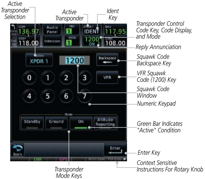
Figure 2-1 XPDR Control Display
