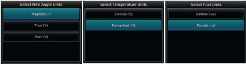
Figure 16-26 Setup Units Selection Windows
