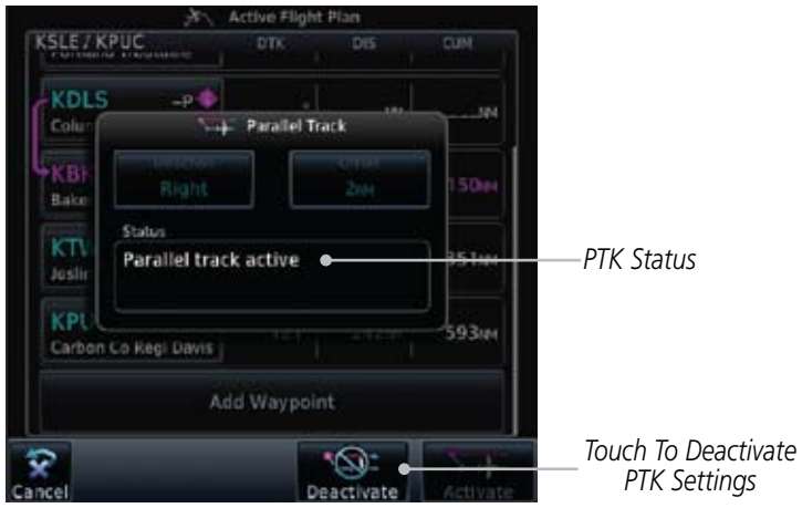
Figure 4-30 Deactivating Parallel Track
