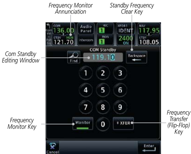
Figure 3-19 Com Frequency Monitoring
