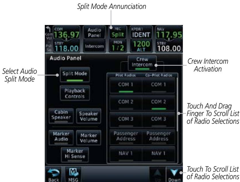
Figure 2-15 Audio Panel Split Mode Controls
