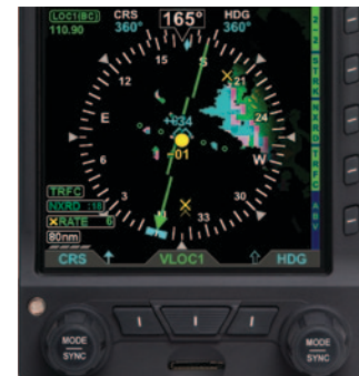
Figure 4-114 Navigation Display Showing Hazard Awareness
