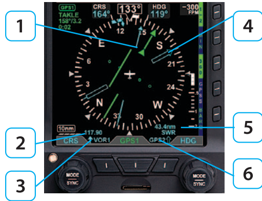
Figure 4-76 Bearing Pointer Description
